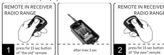
Fig. 5 Remote assigning of the remote in the radio range of the receiver.
