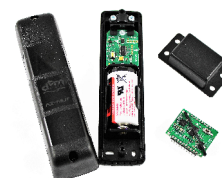
AZYMUT wireless gate status sensor
