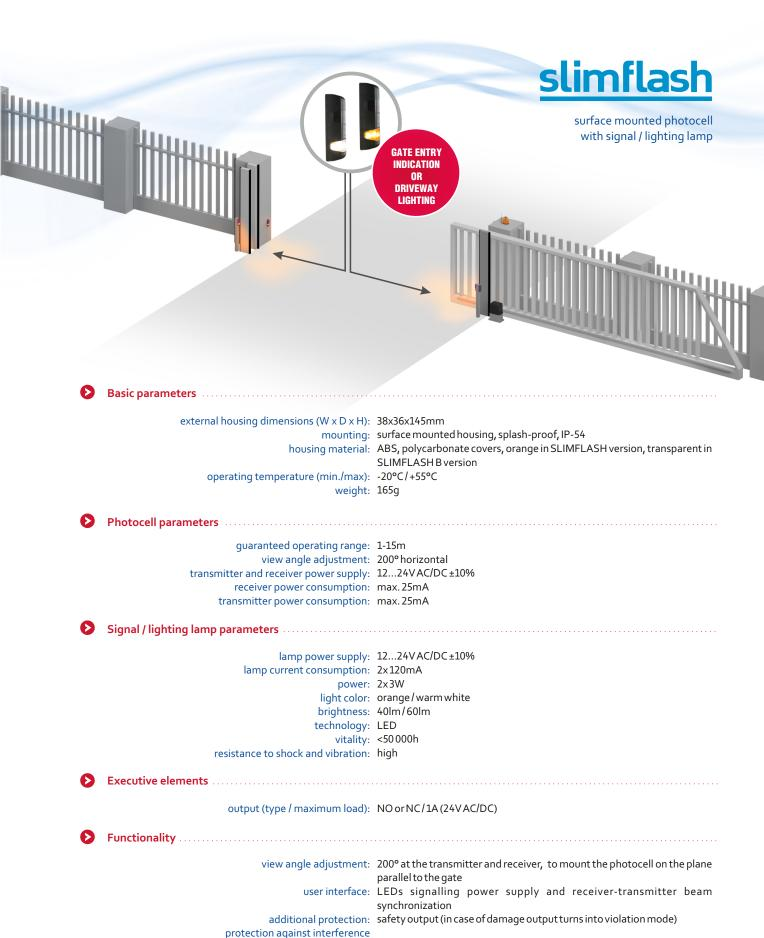
with 2 pairs of photocells: yes, synchronization function (AC supply required)
