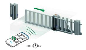
user in receiver radio range initiates adding a transmitter to receiver by using remote buttons, since that moment remote is active in the system
