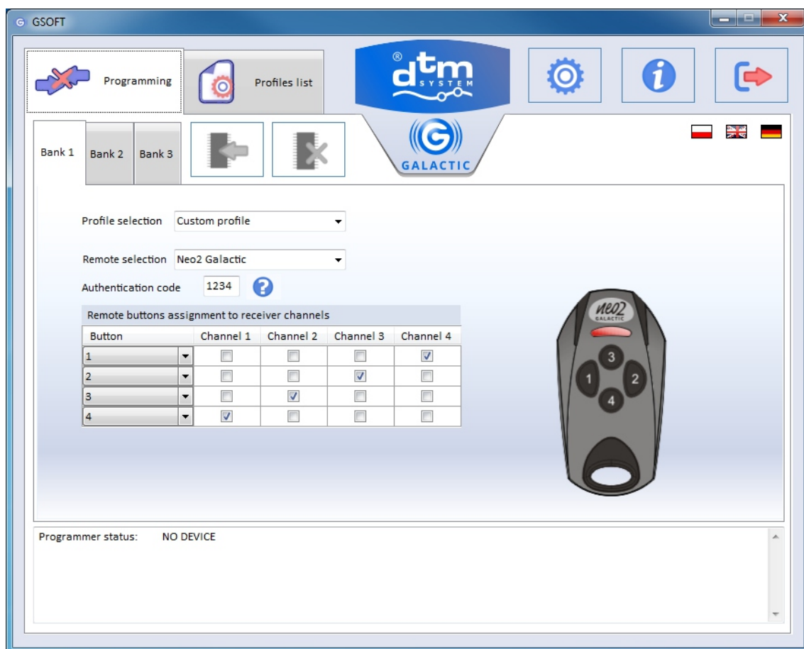
Fig. 3 View of the main window of GSOFT programme with the information about the lack of connection of the GPROG programmer.
